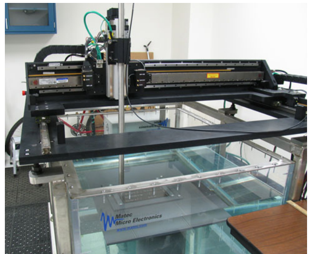
Fig. 5 Ultrasonic scanning tank
